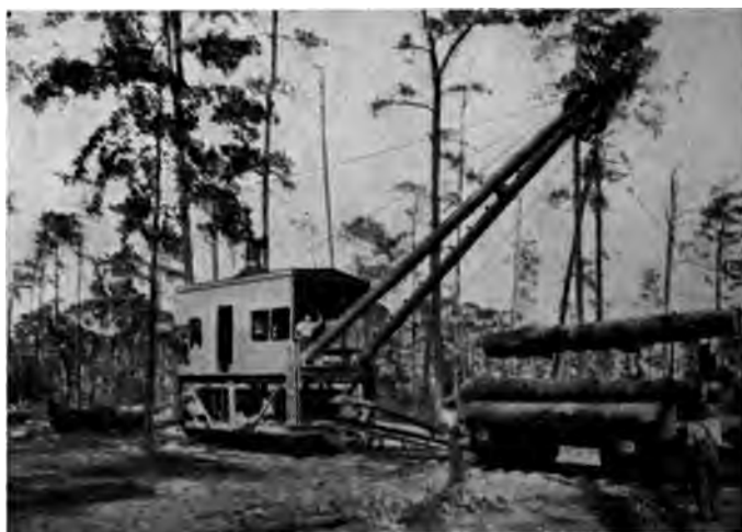
FIG. 94.—A Decker Log Loader.
